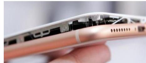
Figure 1: iPhone with Housing Separation
