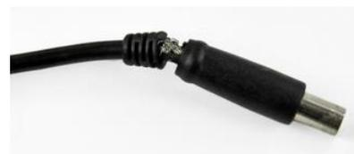
Figure 2: Damaged Laptop Charger
