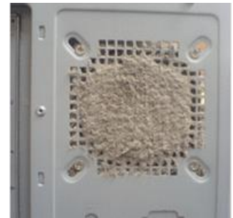
Figure 1: Vent Blocked by Dust
